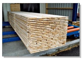
Stacking of mixed widths with side distance
