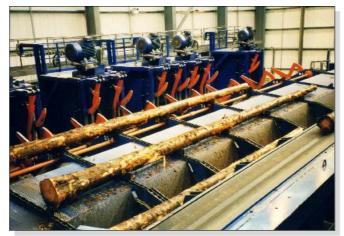
High capacity cross-cutting line for long poles
