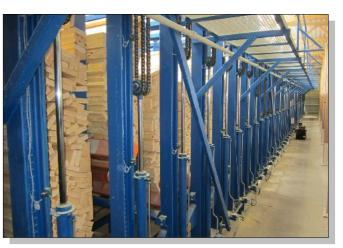
Box sorting line for boards and timber
